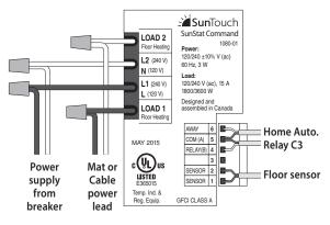
Sensor, relay and home automation connections are made to the terminal block by inserting the wires into the square openings and tightening the screws on the side.
